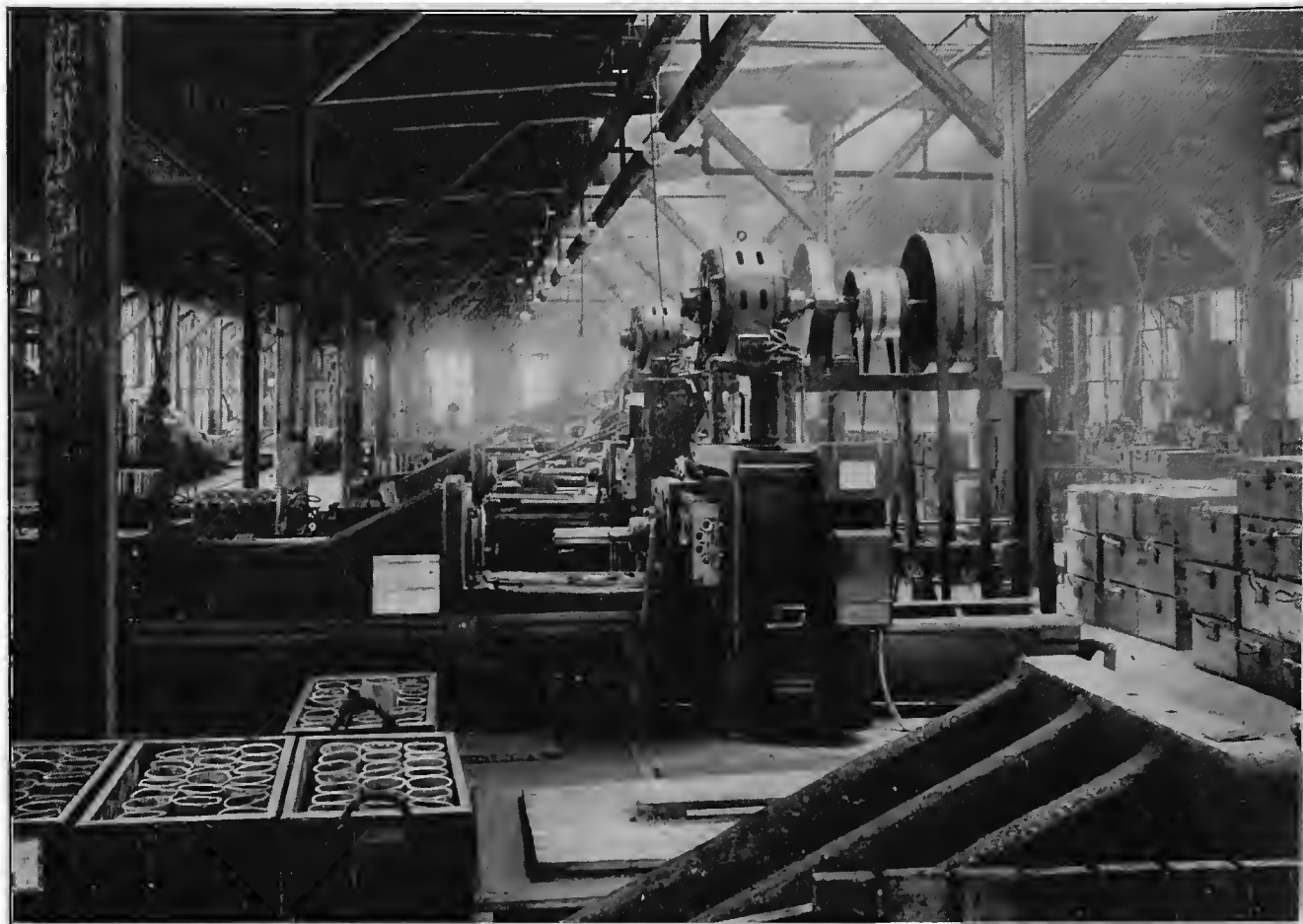
FIG. 9. FROG PLANERS DRAWING BRASS CARTRIDGE CASES
